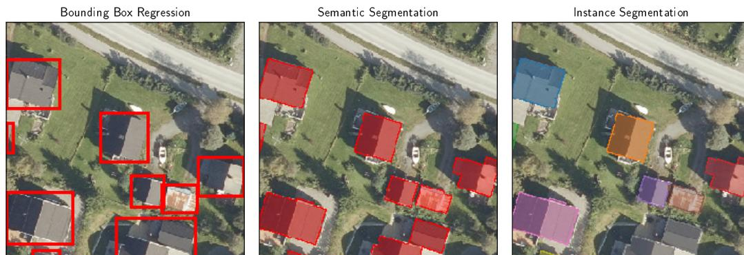
**Figure 2:** Different granularities for single-class building localization, using the Trondheim 2017 data set. Bounding box regression is shown on the left, semantic segmentation in the middle, and instance segmentation on the right.
