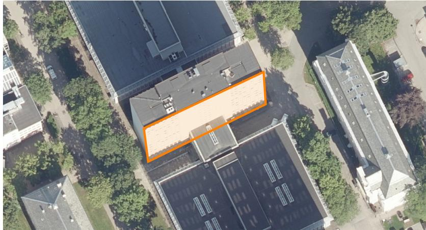
**Figure 16:** Example of nonproper orthophoto. The building centered in the image is 14 stories tall. The orange area annotates a clearly visible building wall. ©Kartverket.
