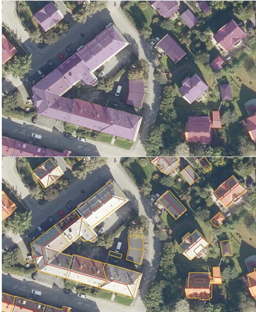
**Figure 58:** **Top** – Low-fidelity building footprint data marked in **purple**. **Bottom** – High-fidelity geometric line segments defined from roof geometries. Ridge lines, for example, are shown in **red**. ©Kartverket.
