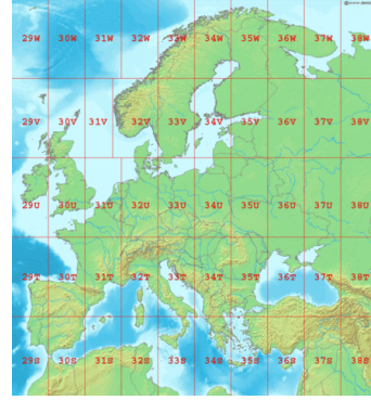
Figure 2.1: The figure shows the UTM zones required in order to cover the entirety of Europe, from 29S to 38W. This public domain image has been sourced from Wikimedia [10].
