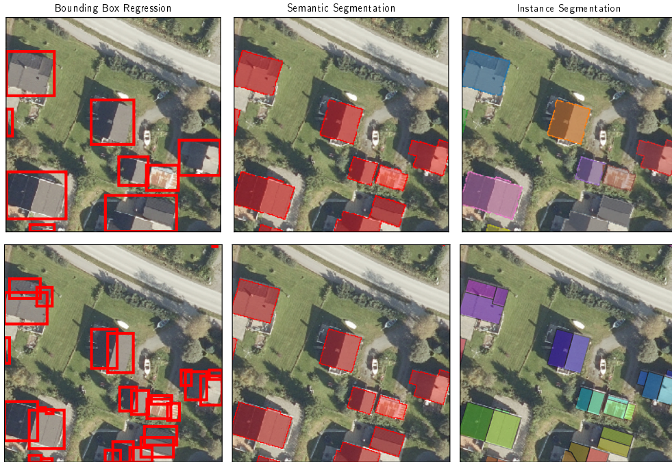
Figure 1.2: Different granularities for single-class construction localization, using the Trondheim 2017 data set. Bounding box regression is shown on the left, semantic segmentation in the middle, and instance segmentation on the right. The top row defines entire buildings as the objects of interest, while the bottom row considers each individual roof surface as distinct objects.
