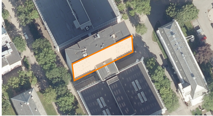
Figure 2.6: Example of nonproper orthophoto. The building centered in the image is 14 stories tall. The orange area annotates a clearly visible building wall. © Kartverket.
